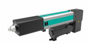
Image 2 shows the EX-K type from the line-X series. Perfect for clinching, riveting, insertion of functional elements, punching and press applications with limited installation space. Press forces 10, 30, 60, 100, 200 kN. Customer-specific configurations are possible, e.g. speed, extension of force holding time, protection class IP65, stroke length ....
