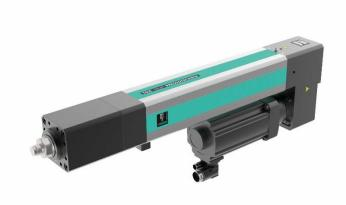
Image 3 shows the EX-F type from the line-X series for press applications with short clock times. Press forces 5, 10, 30, 60, 100 kN. Customer-specific configurations are possible, e.g. speed, extension of force holding time, protection class IP65, stroke length ....
